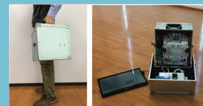
Figure 6 Prototype of the integrated automated portable device. All parts of the device are assembled in a compact 300 mm x 300 mm x 300 mm and 12.8 kg container. The device runs with a 24-V battery power source and is connected to a tablet screen.
